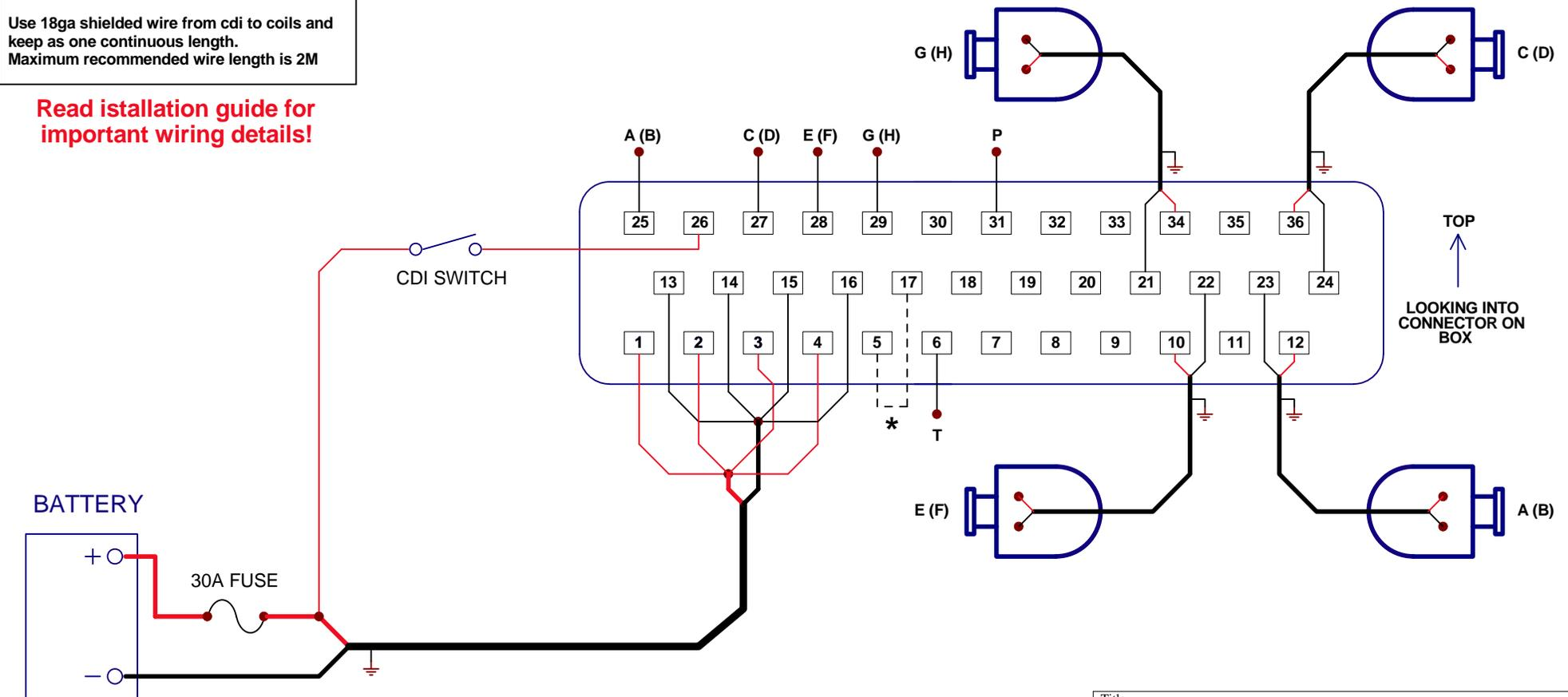
**Reverse polarity connection without fuse installed will damage unit!**
