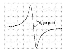
The diagram above shows the oscilloscope trace of a typical reluctor sensor with correct polarity. Triggering occurs on the negative going zero crossing point.
