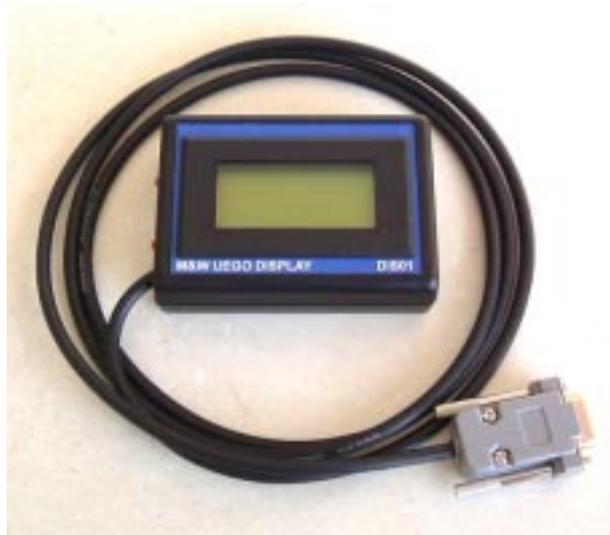
The M&W DIS01 provides a convenient compact display of AFR or Lambda. It connects to the Uego controller via the 9 pin RS232 connector. It needs no external power this is provided by the controller.
