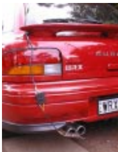
Tail pipe probe has a simple clamp mounting. The cable may be installed through the rear hatch or window.
