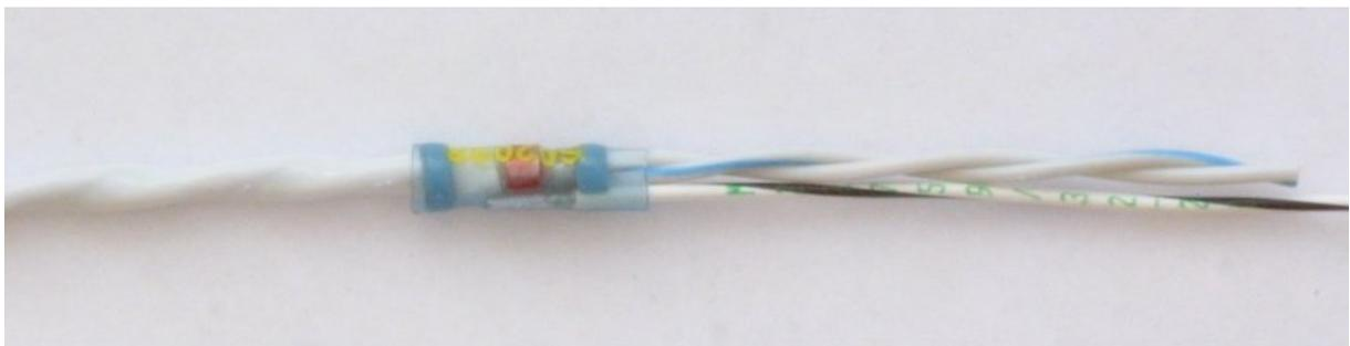
4. Heat shield terminator carefully until the solder ring melts completely and glue is squeezed out both ends sealing the joint. This will usually take an air temperature of about 300 – 350C.
