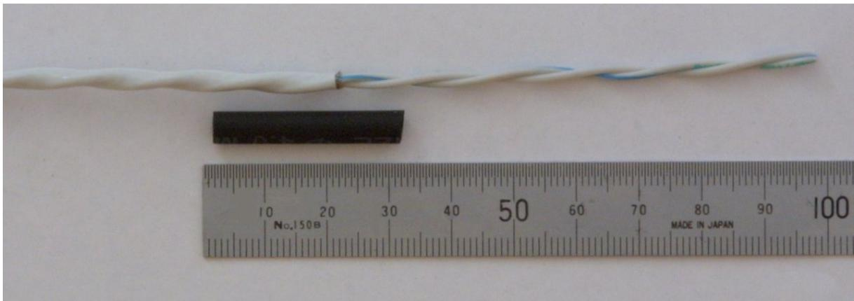
6. Heat the assembly at about 200C until glue is seen to appear at both ends of the joint.
