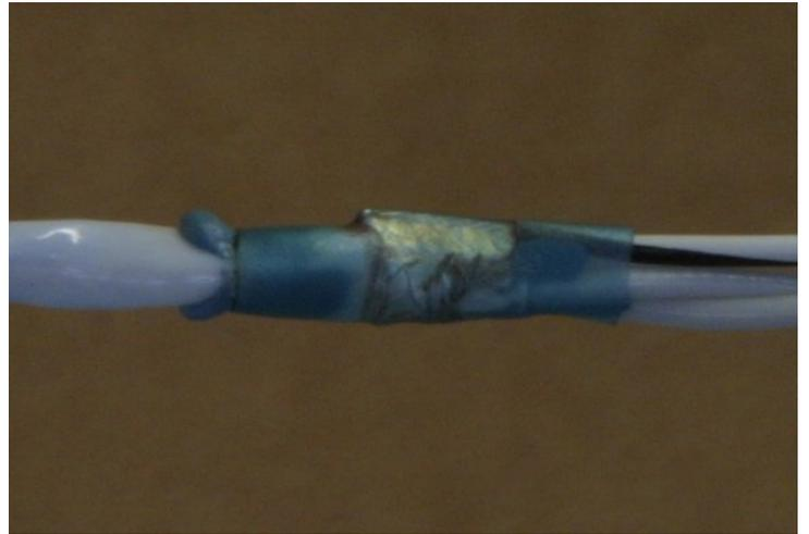
5. To complete the assembly it's necessary to seal the other end against ingress of water. Trim sufficient sheath and completely removing the exposed braid. Take a 30mm piece of 4mm glue lined heat shrink and slip this over the wire so that it covers both shielded and non shielded portions equally.
