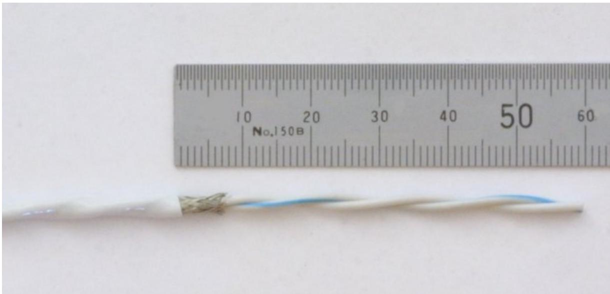
3. Push the shield terminator over the wire ensuring all braid strands pass through the solder ring. This can be achieved by gently rotating the wire while holding the terminator stationary.
